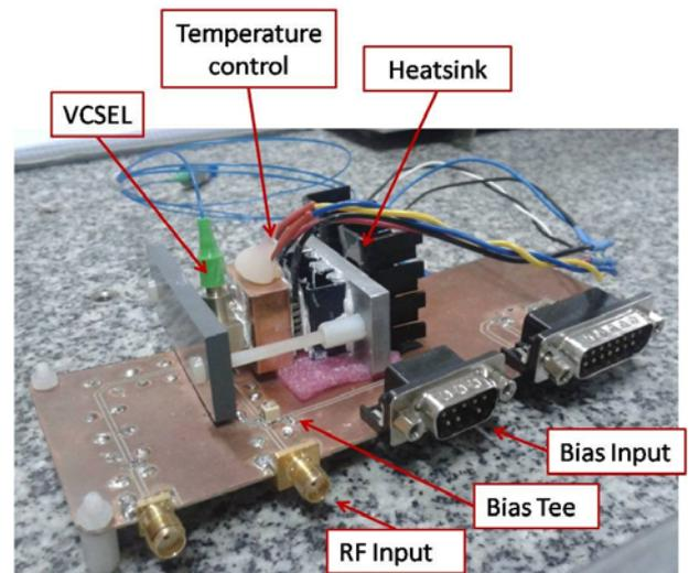
*Vertical-cavity surface-emitting laser (VCSEL) based, optical frequency comb generator (OFCG). Source: Carlos III University of Madrid*
