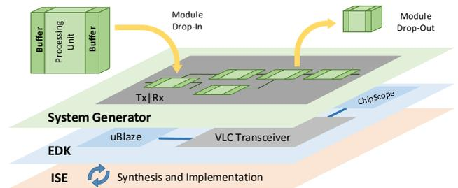
*Software development flow and Xilinx tools used in the VLC test-bed. Source: Aveiro University.*
